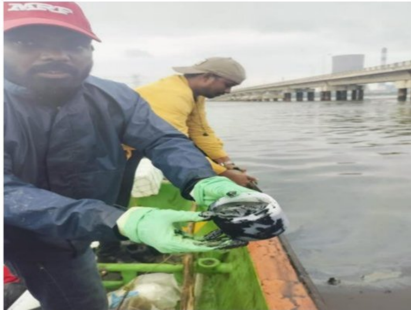
Figure 19: Sediment sample collection from midstream and banks
