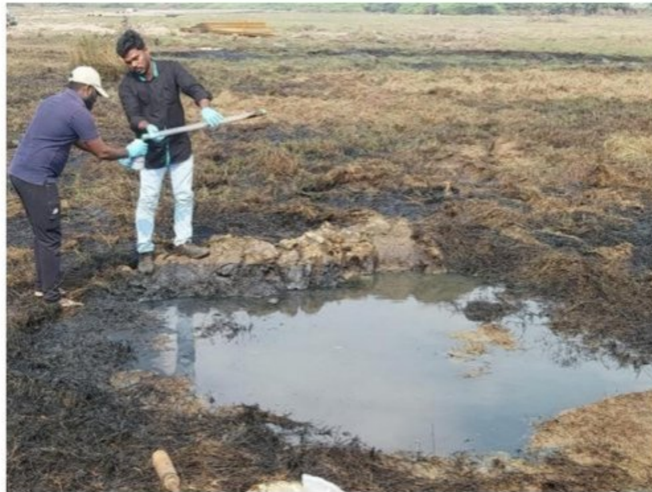
Figure 22: Collecting water samples using a bailer
